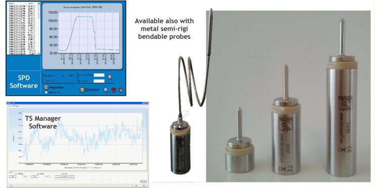
P-Micro and S-Micro are easily employed in the food industry: they can be used in packages, containers, jars or loosely inside pasteurisers to monitor the product temperature at its core, for example in freshly filled-pasta.
