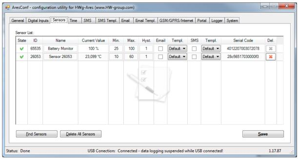
Use this tab to configure basic and advanced properties of sensors:
