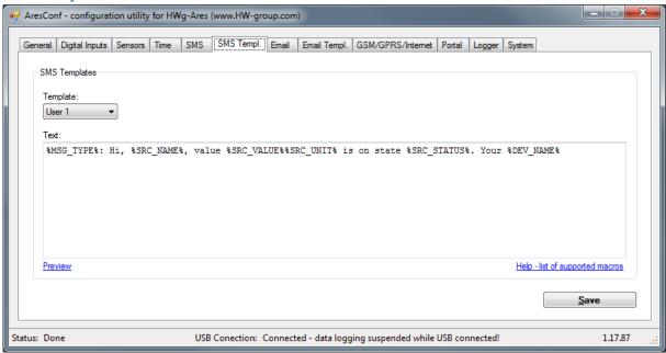
Use this tab to define the formats of individual messages, e.g. to distinguish temperature alarm messages from humidity alarm messages or to define the contents of status and reminder messages.
