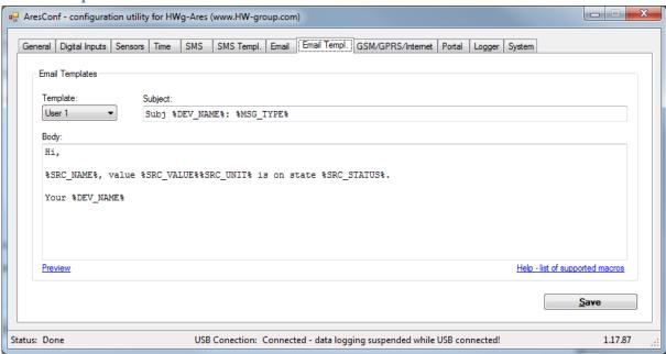
Use this tab to define the format of individual messages, e.g. to distinguish temperature alarm messages from humidity alarm messages or to define the contents of status and reminder messages.
