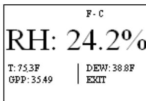
2. **The meter will begin taking readings.** As a default setting the RH reading will be the most prominent on the screen. If you would like to make another variable (temperature, GPP/GPK or dew point), the prominent reading, use the  $\uparrow$   $\downarrow$  and  $\leftarrow$   $\rightarrow$  keys to highlight your selection. Press the **SELECT** key to choose that variable.
