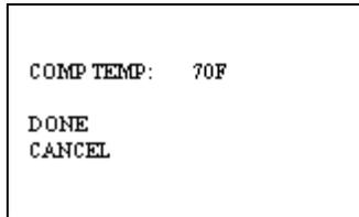
2. **To scroll through the temperature settings**, use the ⇐ ⇒ keys to scroll up or down to a higher or lower temperature value. Temperature values will change in 5°F increments.
