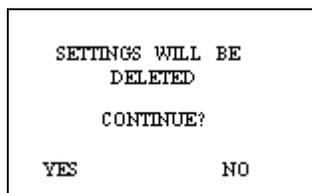
2. **Use the  $\leftarrow$   $\rightarrow$  keys to answer "YES" or "NO."** If you answer "yes," the meter will return to factory default settings in basic mode; i.e. Species = Douglas Fir, Temperature correction = 70 F, Alarm = OFF in pin mode. In Scan mode, Alarm = "off."
