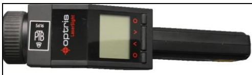
Transfer standard IR thermometer LS-PTB
