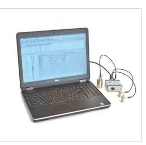
Qlever operating with loggers connected to a Multi USB interface
