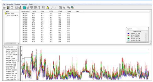
**Real time acquisition window** allows both monitor and recording, in graphic and numeric format. Data are acquired from one of the measuring modes (SLM, Profile, Octave or Third Octave) available on Delta Ohm sound level meters. Data storage can be either on the sound level meter's flash memory, on PC memory or on the both.
