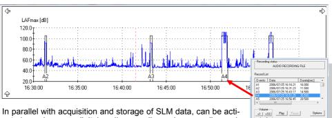
In parallel with acquisition and storage of SLM data, can be activated synchronous digital audio recording using a audio card. Playback of audio tracks can be directly made using Noise Studio interface.
