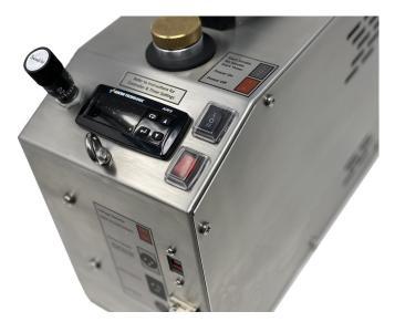
An intelligent PID controller allows operators to adjust temperature ranges to suit different aerosol reagents (Ondina, PAO, DEHS) as well as the ability to set aerosol on / off periods.
