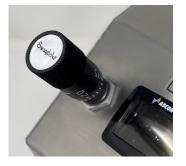
Vernier Scale Adjustment Valve), gives further versatility in terms of adjusting the aerosol output
