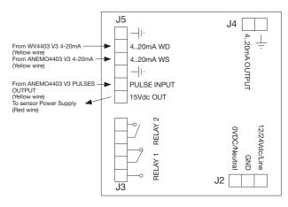
J3: Output relays connector. Configuration through P09 y P16. J4: Analogue output connector. Configuration through P24 y P25. J5: Wind sensors connector. Configuration through P01, P02 y P03.\*
