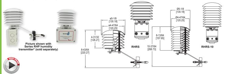
The **Series RHRS Outside Air Humidity Radiation Shields** protects outside air humidity transmitters from rain and radiated heat. With the curved shape and color of the plates, air flow is able to move across the sensor to keep radiated temperatures from rooftops and surrounding surfaces from affecting humidity readings.
