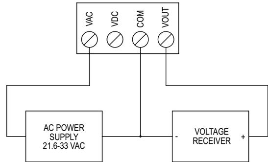
**Figure 3: AC wiring**
