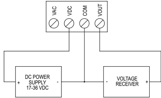
**Figure 2: DC wiring**
