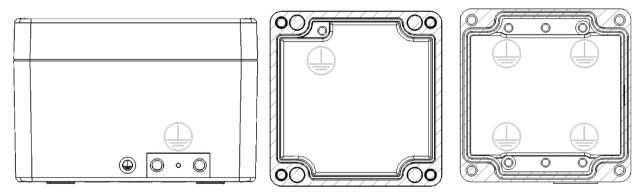
Note that the external and internal earths of the enclosure share an electrical connection, but the lid does not. Both parts of the enclosure must be connected to a suitable ground connection.
