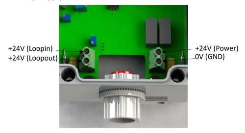
There must be no conductor extending beyond the terminal block, strip wires no more than 10mm.
