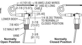
The SERIES V10 Flotect® Mini-Size Flow Switches is designed to provide inexpensive. reliable monitoring of the presence or absence of flow in a system. This series is available for field installation in pipelines from 1/2 to 2" diameter and available in brass or 303 SS body.
