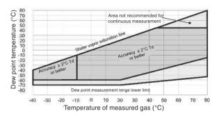
Dew point accuracy vs. measurement conditions
