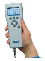
The Vaisala DRYCAP® Hand-Held Dewpoint Meter DM70 is ideal for fieldchecking DMT340 transmitters.
