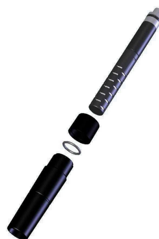
Figure 1. The structure of the in-soil adapter and a GMP222 probe.
