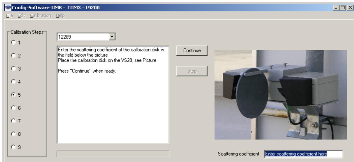
Please input in ,Scattering coefficient' the measurement which is given on the calibration disk (in  $\text{km}^{-1}$ ) and ,Continue'. After 3 more minutes and successful adjustment, finish with ,Stop'.
