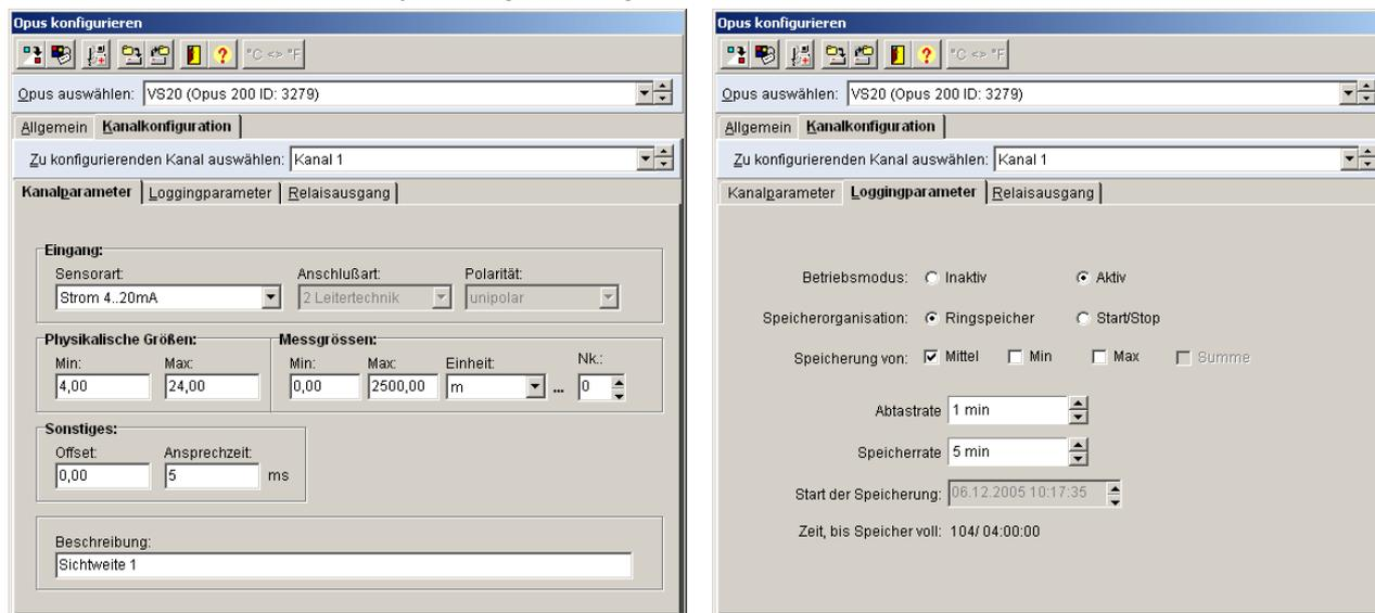
If the current output is scaled to a different value the setting must be adjusted accordingly:
