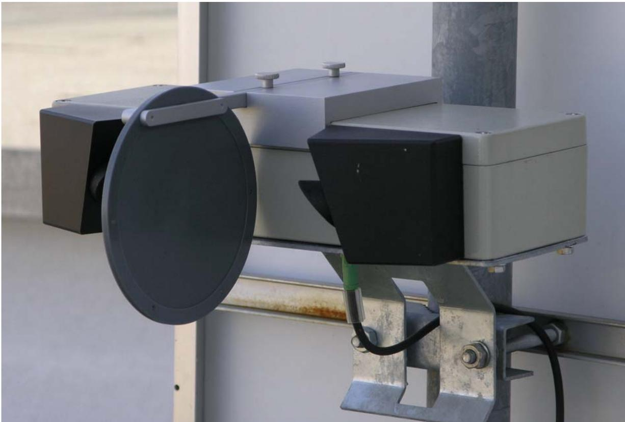
By using software „UMB-Config-Tools“, the visibility can be displayed. Please note: wait at least 2 minutes to get a stable reading.
