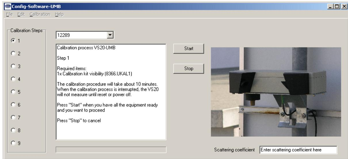
After 3 minutes, the software allows to install the calibration disk.
