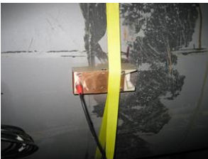
Figure 33: Textile tension bands are recommended for the assembly of the XUC-PW-F05 transducers (temperature limitation)
