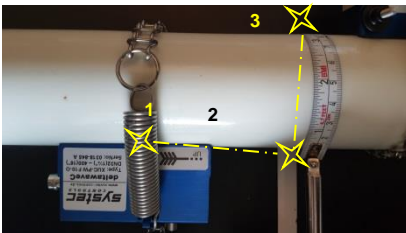
Figure 19: Mark the position of the second transducer at half circumferential distance
