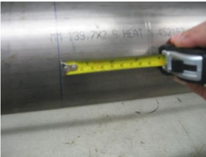
Figure 16: Mark the distance between transducer
