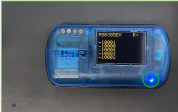
You may now disconnect the Base Station from your PC. It is recommended that you keep your Base Station charging during measurements, as the Autonomous Battery Life is approximately 48 hours; Below the minimum required 72 hours for an ISO 9869 conforming measurement.
