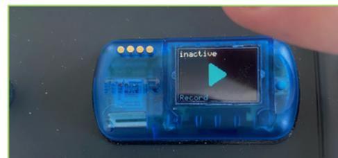
**Hold down** the toggle button to see other menu options, and release to go to highlighted option. For instance, if you want to exit the main menu, and go to recording options. Hold down the toggle button until "**Record**" is highlighted, and let go of the toggle button to move to this page.
