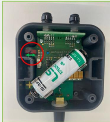
Change the Frequency of Measurements by alternating the Switch circled above
