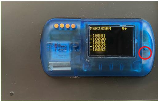
Used to navigate Base Station interface.
