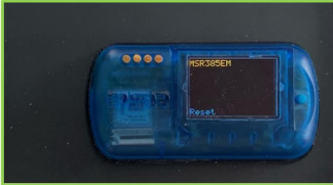
Resets Nodes registered on Base Station Press once to Reset. Hold down button for option to cancel.
