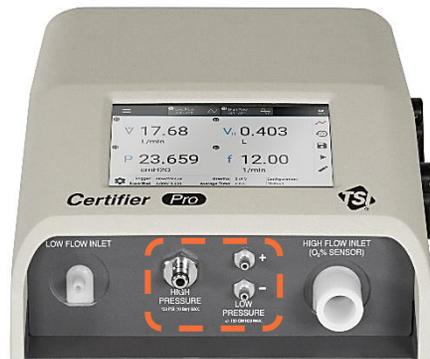
2. Press the zero icon located in the right navigation bar of the Certifier™ display (see below right).
