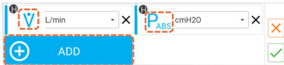
Once pressed, a list of available measurements will be displayed in alphabetical order (see below left). An H is displayed in the upper left to indicate the measurement is coming from the high flow channel, and an L is displayed for measurements coming from the low flow channel. Swipe up and down to scroll through the list options, tap to select.
