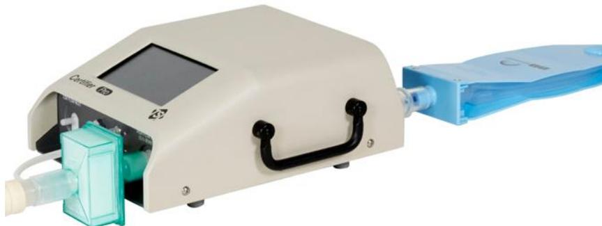
7. Configure the Certifier Pro Flow Analyzer settings from the instrument display as specified by the manufacturer of the device under test. A Certifier Flow Analyzer user configuration could be loaded if available.
