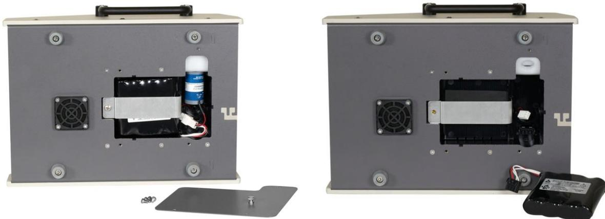
To install a battery into the Certifier™ Pro Flow Analyzer:
